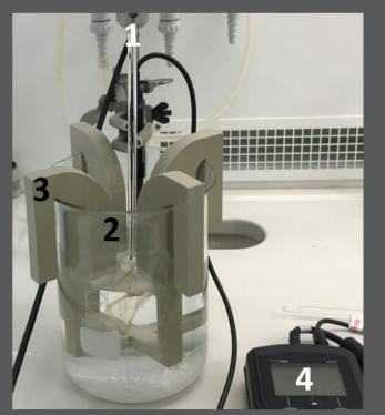
Precipitation reactor consists of a curved blade (1) connected to a rotor; a 2 L decanter glass (2); stators (3); and a pH-meter (4)
