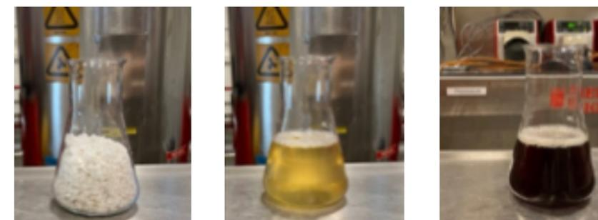
Figure 2. Fibre sludge (left) has been converted to hydrolysate (middle) through enzymatic hydrolysis. The hydrolysate has been used in lactic acid fermentations (right)
