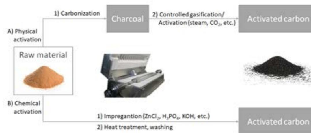
Figure 26. The preparation process of the activated carbon by physical or chemical activation (Kupila, 2021)
