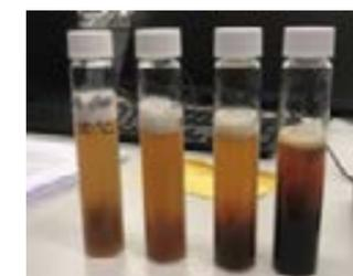
Figure 35. Four consecutive 30 % ethanol(aq) ASE-extracts of spruce bark. Extraction temperature from right to left: RT, 40 °C, 60 °C and 80 °C. Amount of condensed tannins in extracts from left to right: 1.99, 2.74, 5.65 and 34.13 mg/g of dry bark
