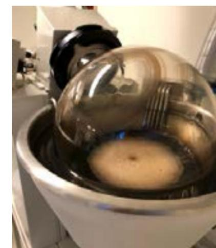
Figure 32. Tannin extract in rotary evaporator
