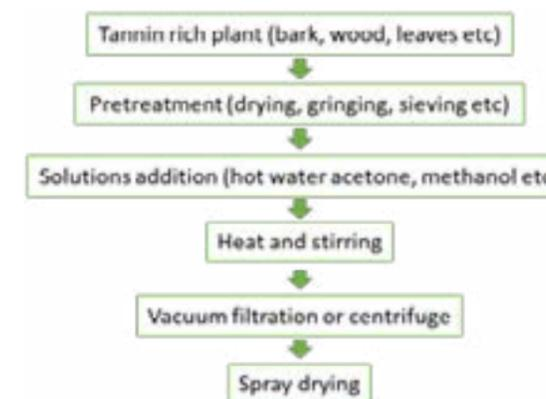
Figure 29. Schematic extraction process to get tannin powder (Adapted from: Shirmohammadli et al. 2018)
