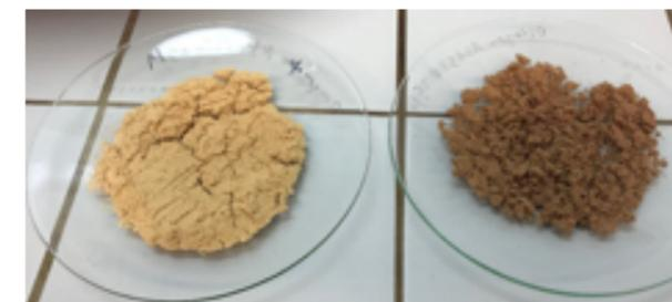
Figure 38. Condensed tannins adsorbed on to Divergan RS®. On the left 2 % NaHSO<sub>3</sub> + 2 % Na<sub>2</sub>CO<sub>3</sub>(aq) extract and on the right 30 % ethanol(aq) extract from ASE-extractions
