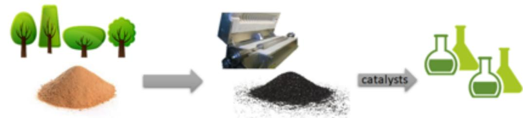
**Figure 16.** Upgrading of the hydrolysis lignin to activated carbon and usage as catalyst support in the biochemical production (Kupila, 2021)
