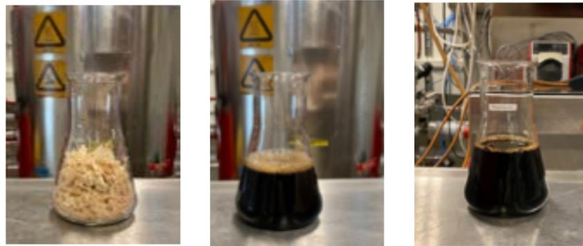
Figure 3. Saw dust (left) has been converted to hydrolysate (middle) through pretreatment and enzymatic hydrolysis and has subsequently been used to produce lactic acid (right)
