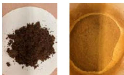
Figure 25. Hydrolysis lignin before (left) and after oxidation (right)
