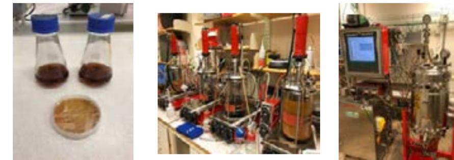
Figure 5. Lactic acid fermentation has been performed in scales from shake flasks (left) to laboratory scale bioreactors (middle) and 50L pilot scale (right)
