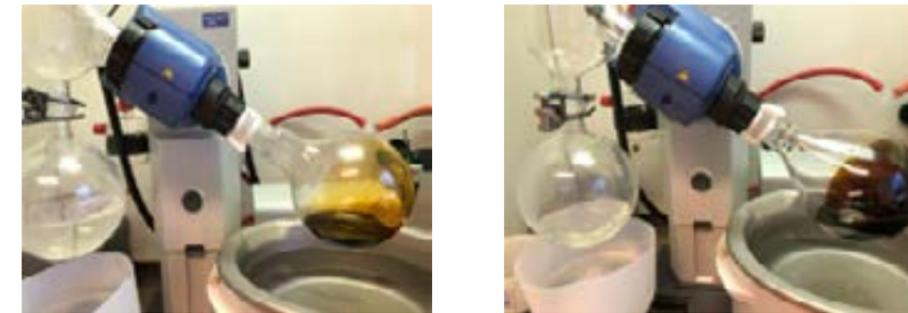
Figure 14. Water removal (left) and distillation of lactate ester (right) from fermentation broth (saw dust) containing lactic acid
