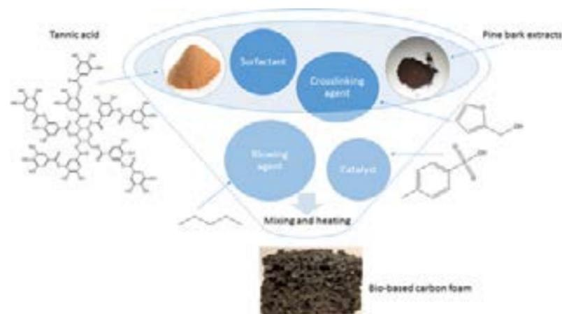
Figure 43. Preparation of the skeletal backbone for carbon-foam support materials using either tannic acid or pine bark extracts. (Varila, T; Mäkelä, E. et al, 2020) Reprinted with permission from Elsevier
