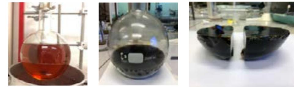
Figure 15. Roughly 50% pure lactic acid (left) produced from fermentation broth (fibre sludge). PLA (middle & right) produced from the pure lactic acid
