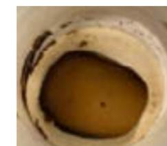
Figure 18. Hydrolysis lignin after washings with the moderately polar solvent tetrahydrofuran
