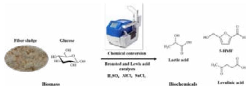
**Figure 13.** Chemical conversion of biomass to biochemicals in microwave reactor catalyzed by Brønsted and Lewis acids. Water was used as the solvent
